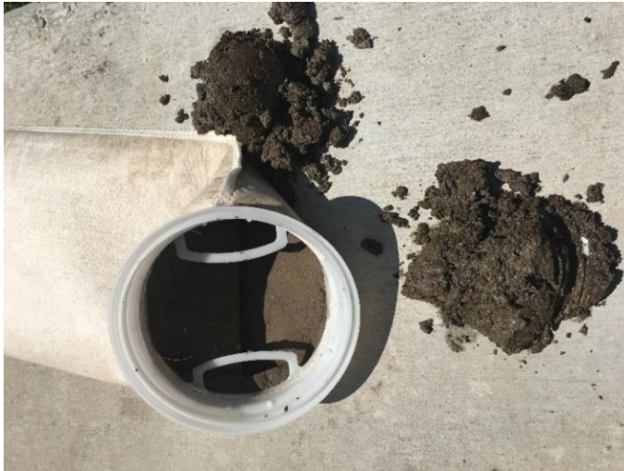
SAND & FOULANT ON BAG FILTERS
